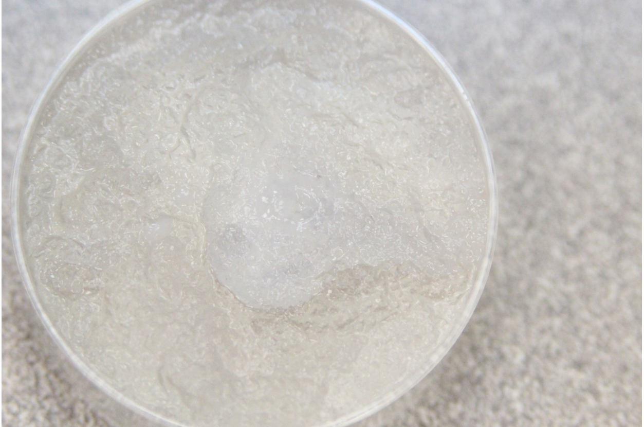
Figure 3.1: Gelatin slurry used in Freeform Reversible Embedded Suspension of Hydrogels (FRESH) printing
